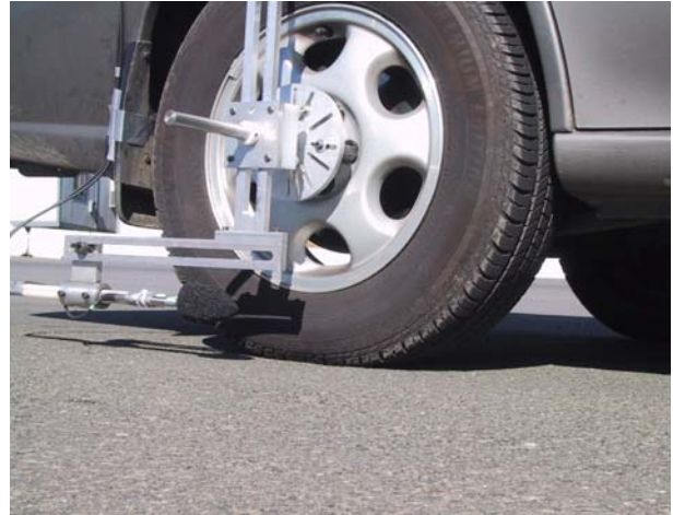
Figure 6.6 CPI measurement illustrating intensity measurement positions (Photo provided by Paul Donovan, Illingworth and Rodkin, Inc.)
