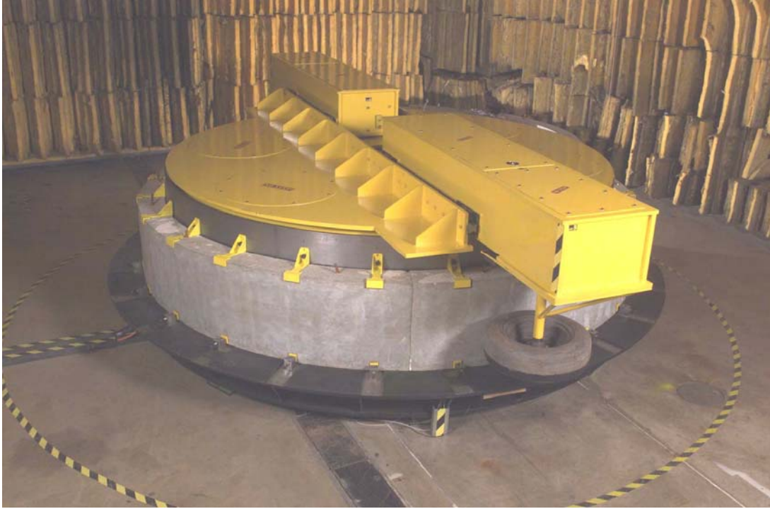
Figure 6.9 Tire/Pavement Test Apparatus (TPTA) with PCC samples mounted on the measurement surface
