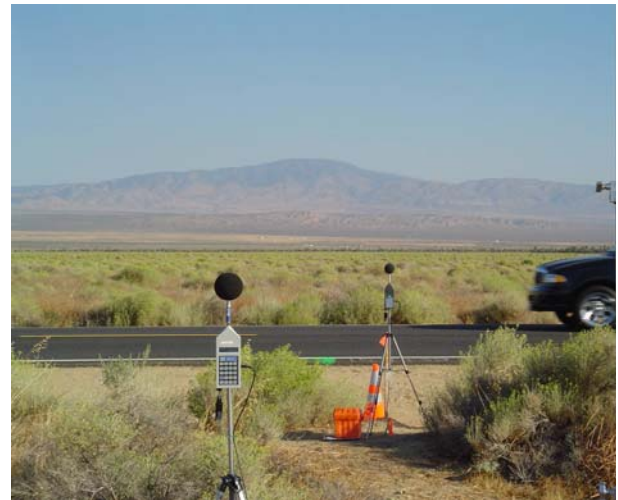
Figure 6.2 Typical measurement set up for SPB measurement. In this case both 7.5 m and 50 ft. measurements are made (Photo provided by Judith Rochat, U.S. DOT Volpe Center)
