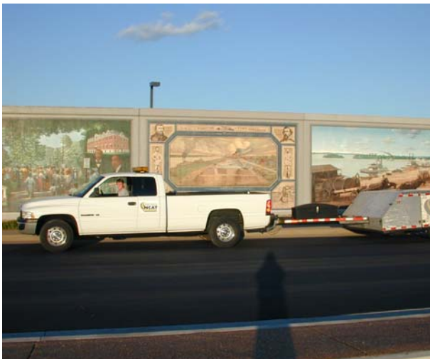
Figure 6.5 Typical CPX trailer measurement (Photo supplied by Doug Hanson, National Center for Asphalt Technology, Auburn University)
