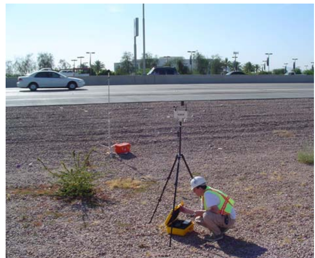
Figure 6.4 Typical measurement setup for a time-averaged sound pressure level measurement (Photo provided by Judith Rochat, U.S. DOT Volpe Center)
